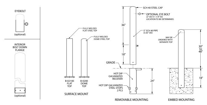
B-2 Bollards shown above in 5" pipe, also available in 8" dia. and in 30", 36", 42", and 48" heights, removable bollard receivers sold separately.
